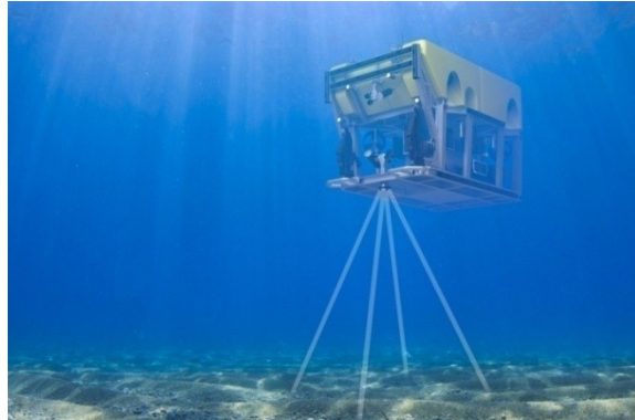
Figure 8: ROV positioning using Doppler Velocity Log and inertial navigation system (Nortek, 2018)
