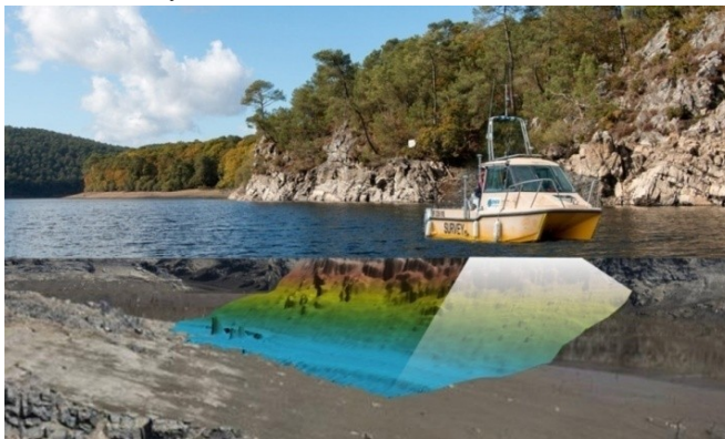
Figure 15 : Bathymetric survey of lake (ENSTA Bretagne, 2018)
